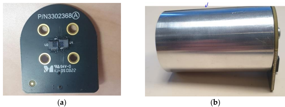
Figure 2. Image of the DUT sample (a) with two sensors; (b) packaged within a metal tube.
