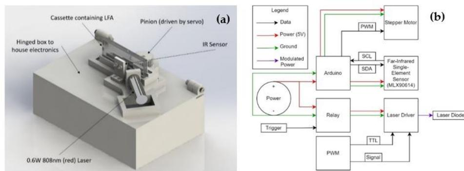
**Figure 2.** (a) Rendering of the device (b) Electronic system overview featuring the laser and motor control systems, and sensor sampling scheme.
