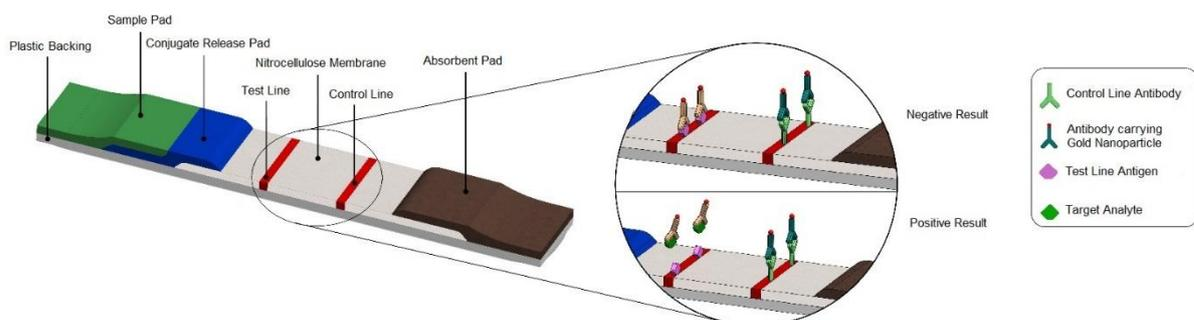
**Figure 1.** A competitive style LFA where the presence or absence of target analyte either blocks or allows binding of antibodies to the antigens in the test line.
