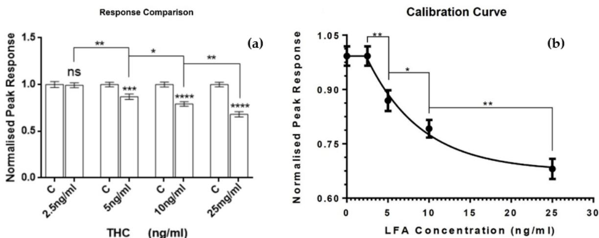
**Figure 4.** Results of 10 repetitions per LFA (N = 20 per concentration) (a) Control line versus normalized test line response (b) Normalized responses fit to a quadratic curve.
