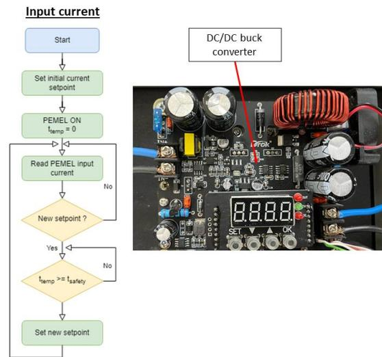
Figure 5. Control algorithms for PEMEL input current. Related DC/DC converter.
