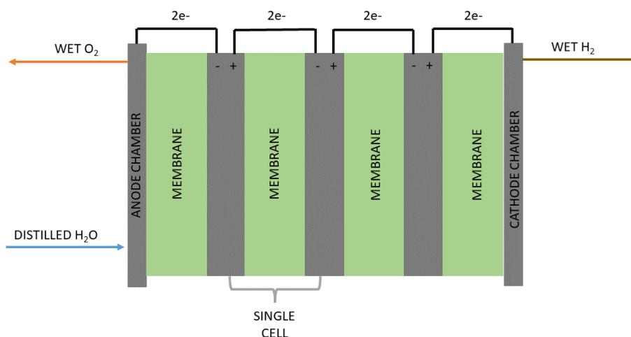
Figure 1. Structure and operation of PEMEL.
