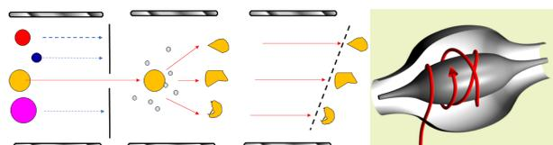
Figure 2. Representation of triple quadrupole and orbitrap analyzers.
