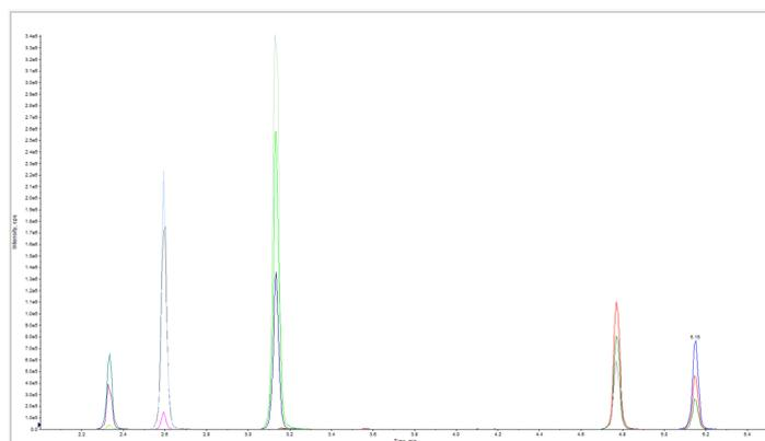
Figure 3. Multiple reaction monitoring extracted ion chromatogram of URB compounds. Chromatographic gradient separation was performed on a 50 x 2.1 mm KINETEX EVO 1.9  $\mu$ m C18 column through mobile phases composed by 0.1% formic acid and 0.1% formic acid in acetonitrile with 5% water. Total run time was 11 minutes at the constant flow rate 0.5 mL/min and the column temperature was set at 40 °C.
