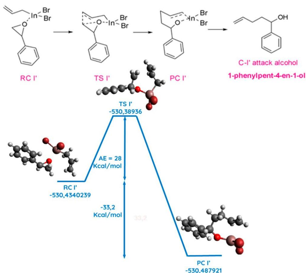
**Scheme 7.** Representative structures (**top**) and Potential Energy Profile (kcal/mol) at B3LYP/LanL2DZ level for the formation of 1-phenylpent-4-en-1-ol (**bottom**).
