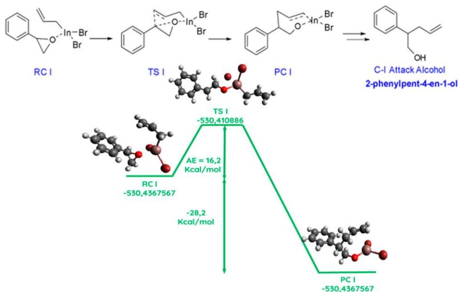
**Scheme 6.** Representative structures (top) and Potential Energy Profile (kcal/mol) at B3LYP/LanL2DZ level for the formation of 2-phenylpent-4-en-1-ol (bottom).
