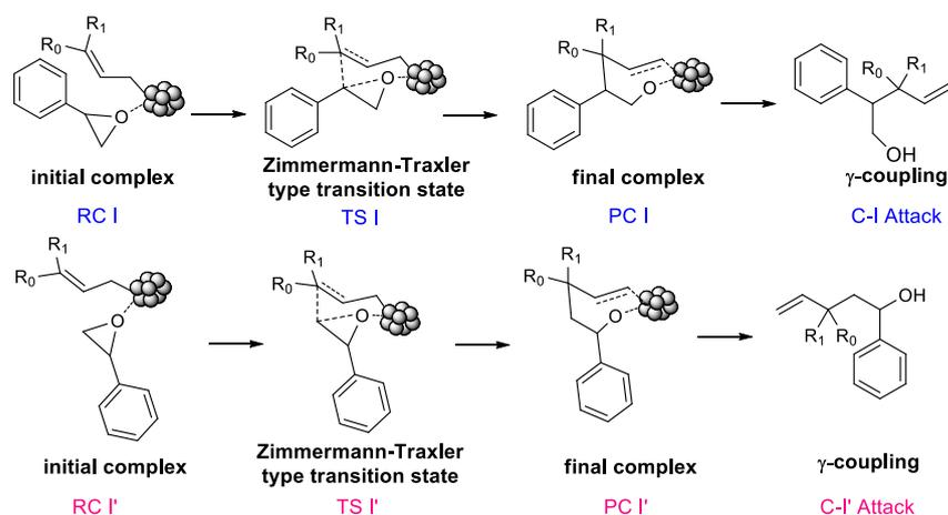
**Scheme 5.** mechanism of formation of both alcohols.
