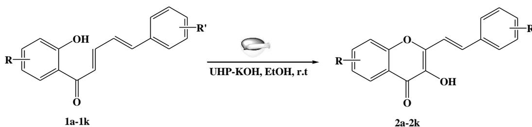
**Scheme 1.** Synthesis of 3-hydroxy-2-styrylchromones using grinding technique.
