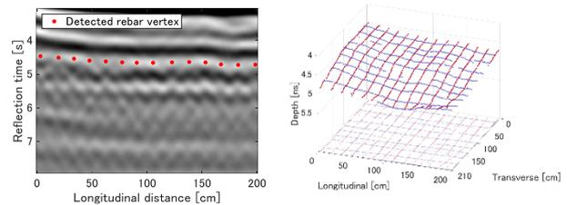
The proposed method was also effective for an in-service bridge data that was acquired 7 cm interval in the longitudinal direction.
