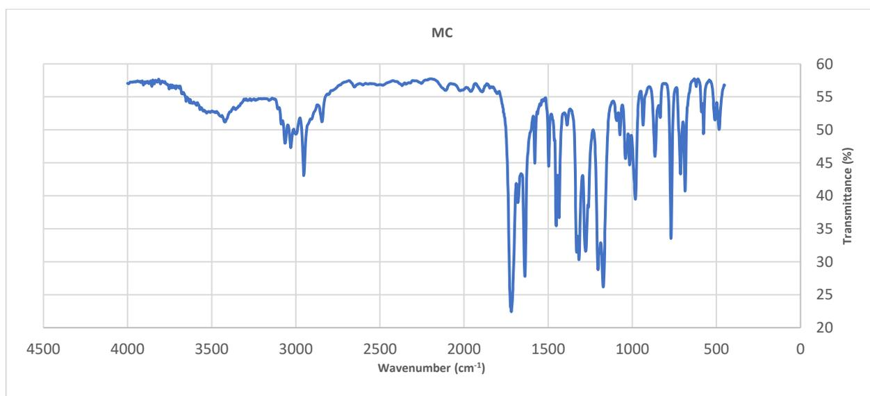
Figure 2. The IR spectrum of methyl cinnamate.
