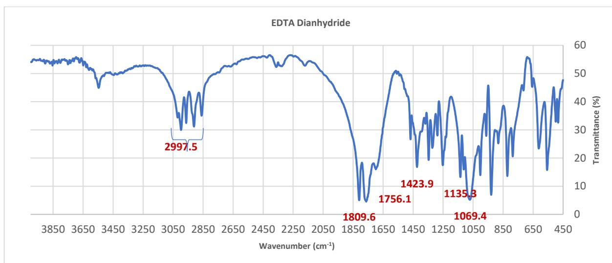
Figure 1. The IR spectrum of EDTA dianhydride.
