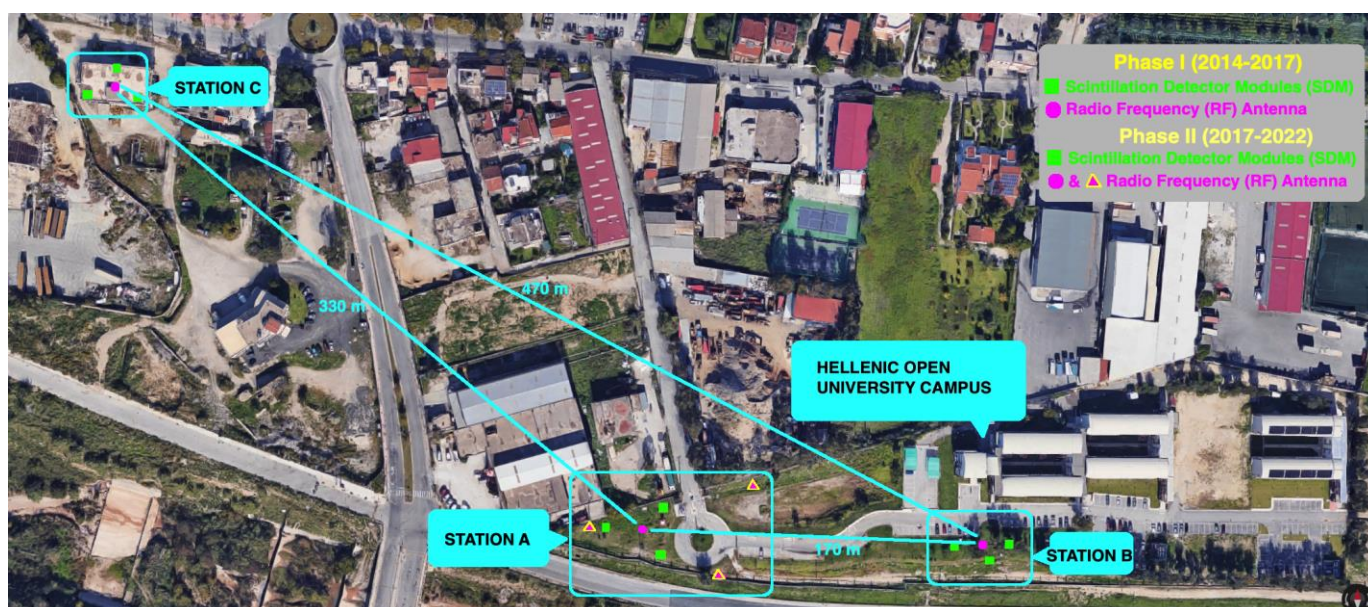
Figure 1. The Astroneu array during its two phases of operation installed at the HOU campus. The positions of the SDMs are marked with green squares, while the positions of the RF antennas with magenta circles. The triangles represent the 3 additional RF detectors installed in station A during the second phase of operation.
