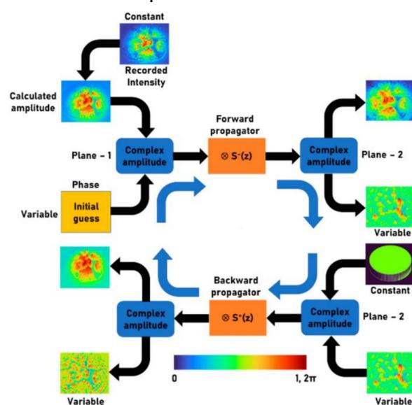
Figure 2 Schematic of the phase-retrieval algorithm[4]
