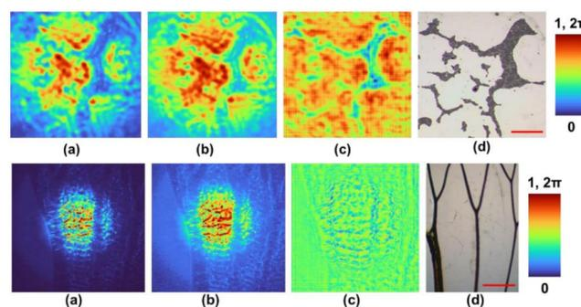
Figure 3: phase imaging results of both latex beads sample (top) and insect wing sample (bottom): (a) Intensity image, (b) amplitude image, (c) phase image, and (d) reference image of the bead samples. [4]
