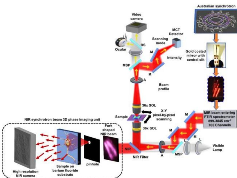
Figure 1: Schematic of the Australian synchrotron's IRM system and the attached synchrotron NIR phase imaging module (shown in the dotted line box). [4]
