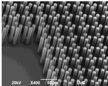
Figure 1: SEM image of the metasurface coated with silver via chemical procedure, showing the resolution of MPL method.
