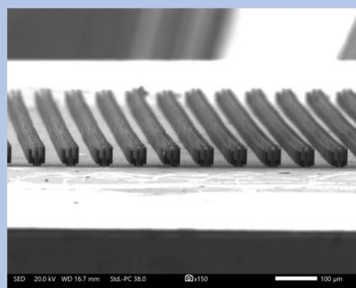
Fig 2. SEM image of fabricated metamaterial.
