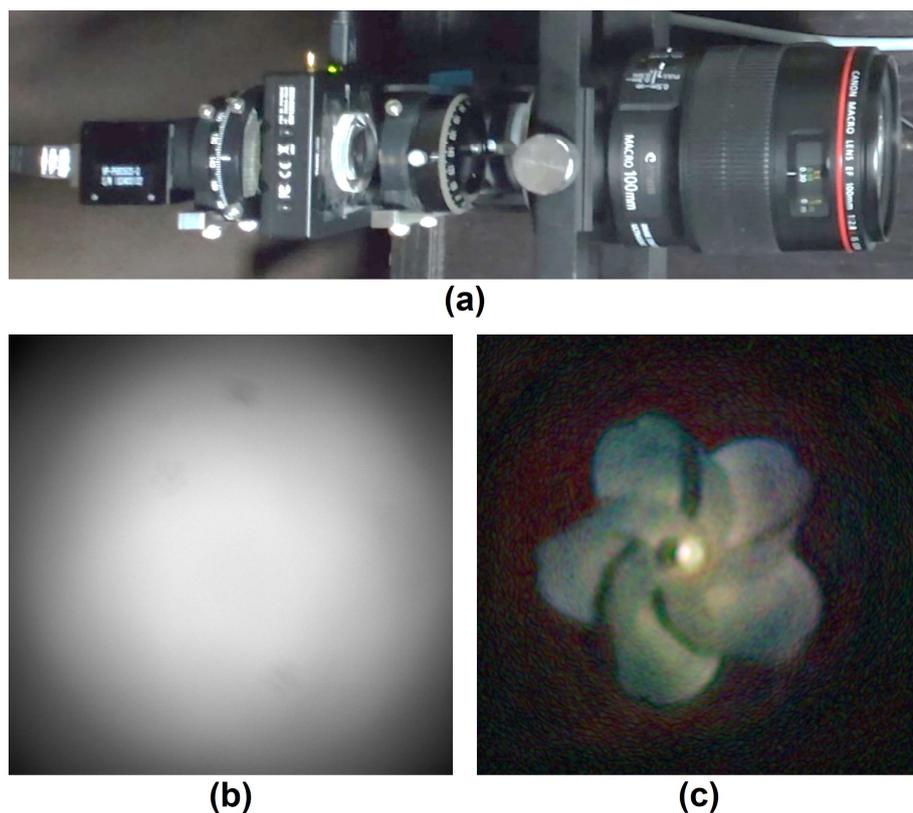
**Figure 2.** An optical implementation and an example of experimental results. (a) Constructed single-shot full-color IDH system with birefringent materials with a camera lens, termed “Holocamera.” (b) A recorded hologram with a holocamera and (c) the image reconstructed from (a).
