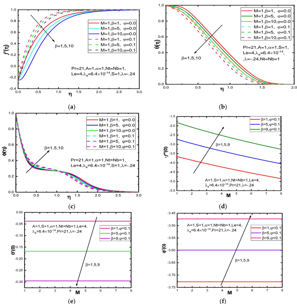
**Figure 2.** Variations of ferromagnetic interaction parameter on (a) velocity; (b) temperature profiles. (c) concentration profile; (d) skin friction coefficient. (e) rate of heat transfer; (f) local Sherwood Number.
