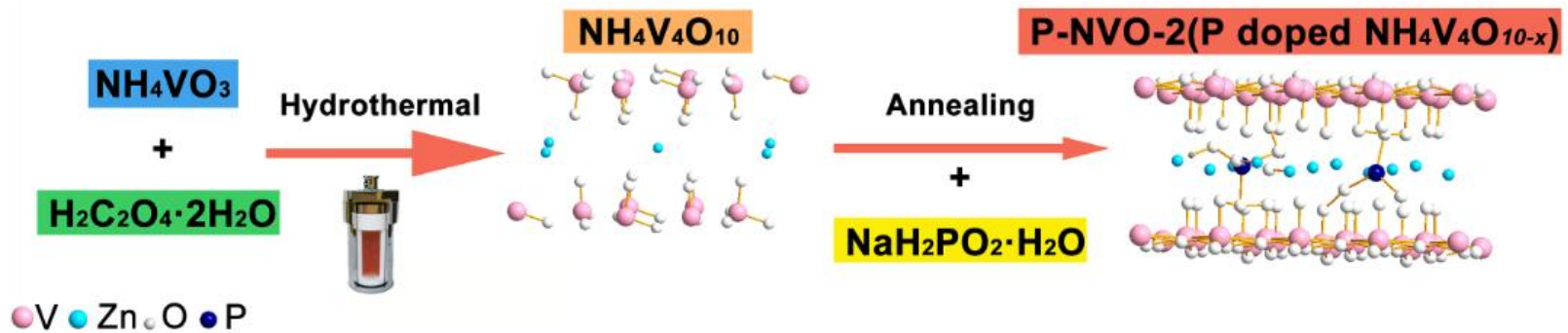
Scheme 1. Schematic diagram of preparation of NH 4 V 4 O 10 (NVO) and phosphate to P-NVO-2.
