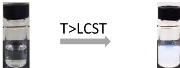
Figure 2. The photographs of nanogels at below and above the low critical solution temperature.
