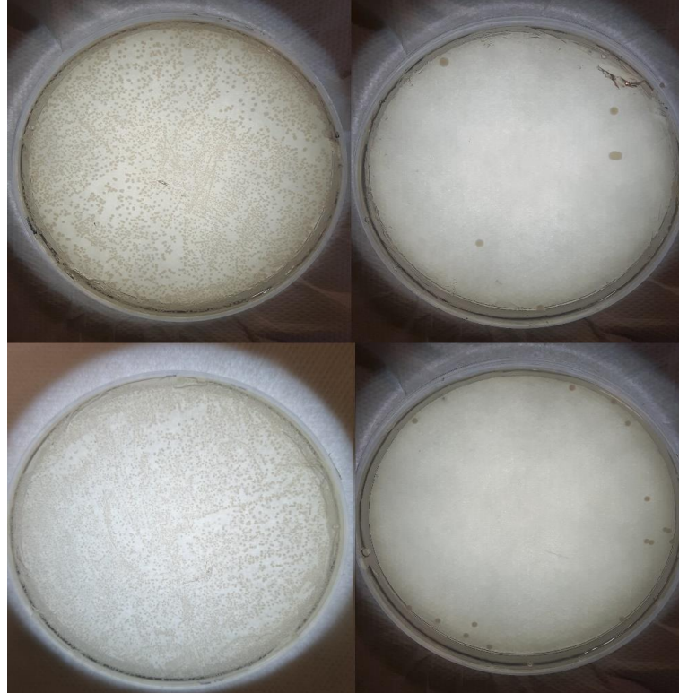
Figure 3. Agar spread plates of E. coli (top) and S. aureus (bottom). The leftmost photos were cultured on uncoated QCM-D crystals, whilst the rightmost photos were cultured on (Naf/CDot) 6 coated discs. Each control-test pair is taken at the same dilution.
