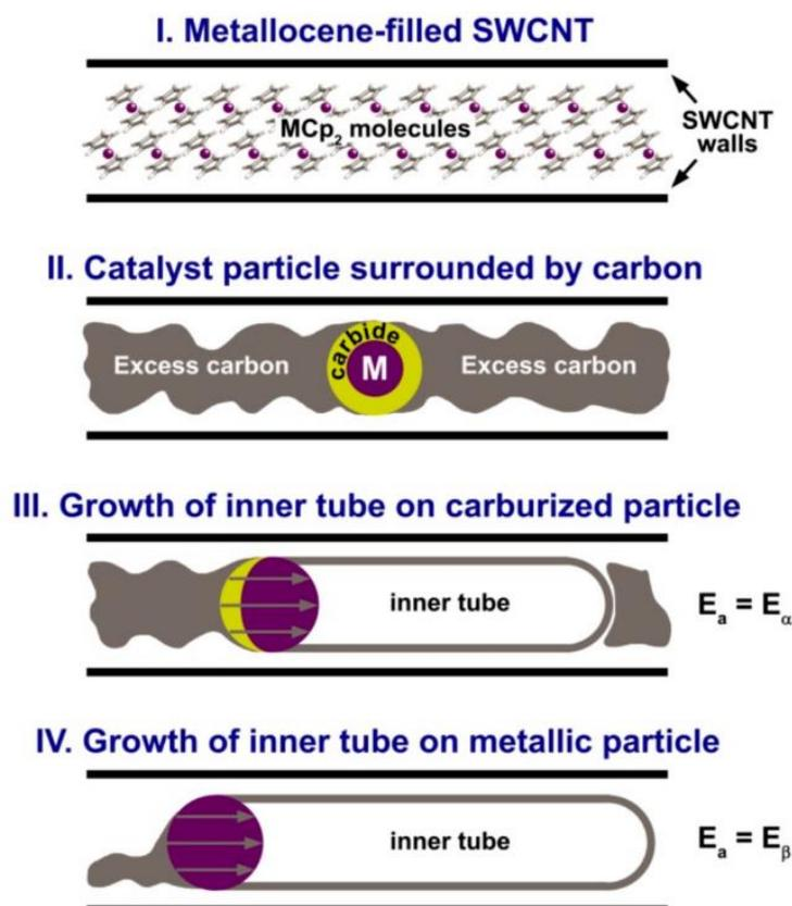
**Figure 1.** Illustration of the growth model of the inner tubes inside the metallocene-filled SWCNTs. MCp2 (M = Ni, Co) molecules encapsulated into the channel of SWCNT. Copyright 2021 by the authors. Licensee MDPI, Basel, Switzerland. This article is an open access article distributed under the terms and conditions of the Creative Commons Attribution (CC BY) license [12].
