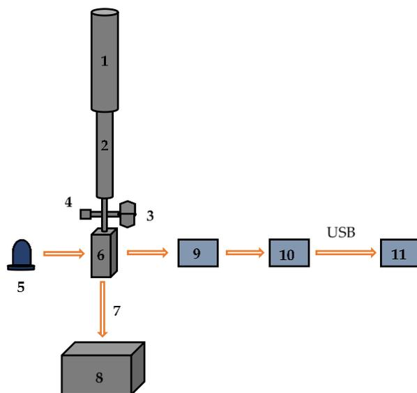
**Figure 1.** The scheme of the optical sensor: 1—LabMate buffer reservoir; 2—PD-10 column; 3—three-way valve; 4—service port; 5—UV LED (255–265 nm); 6—flow cell; 7—flow rate regulator; 8—drain vessel; 9—photodetector; 10—electronic unit, 11—laptop PC.
