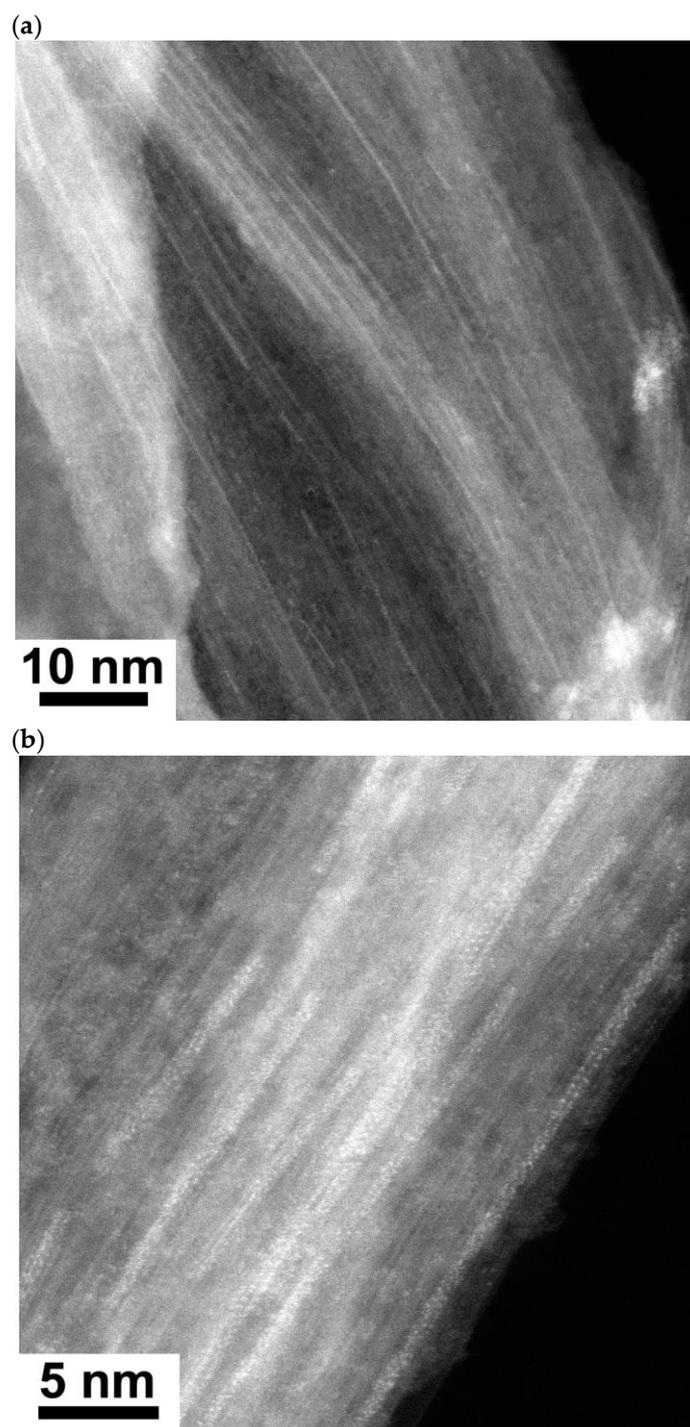
**Figure 1.** The HRTEM image of bundle of lead chloride-filled SWCNTs (a), the image showing individual lead chloride-filled SWCNT (b).
