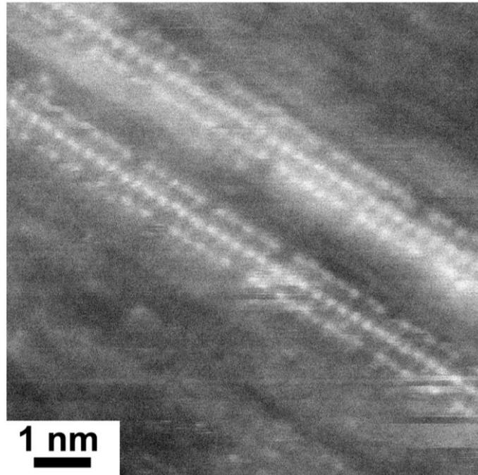
**Figure 2.** The HRTEM image showing two individual lead iodide-filled SWCNTs.
