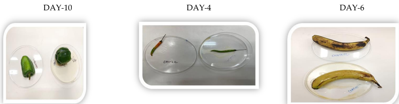
Figure 5. Shelf life improvement properties of pectin + gluten + castor oil films.
