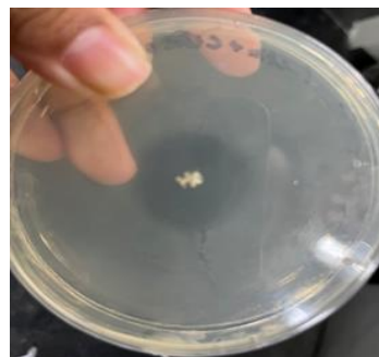
Figure 6. Antimicrobial properties of pectin + gluten + castor oil films with clove oil.
