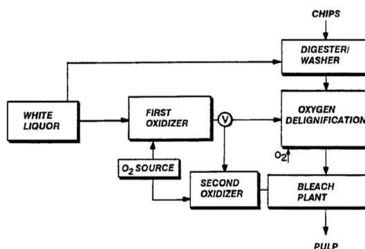
**Figure 1.** Schematic depiction of white liquor oxidation technology integration in a paper mill. Source: Own elaboration.
