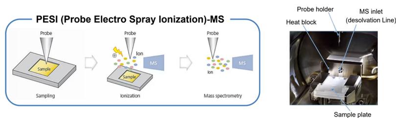
In the DPiMS QT, the sample adhering to the probe surface is ionized by applying a voltage to the probe tip and then introduced directly into the mass spectrometer.
