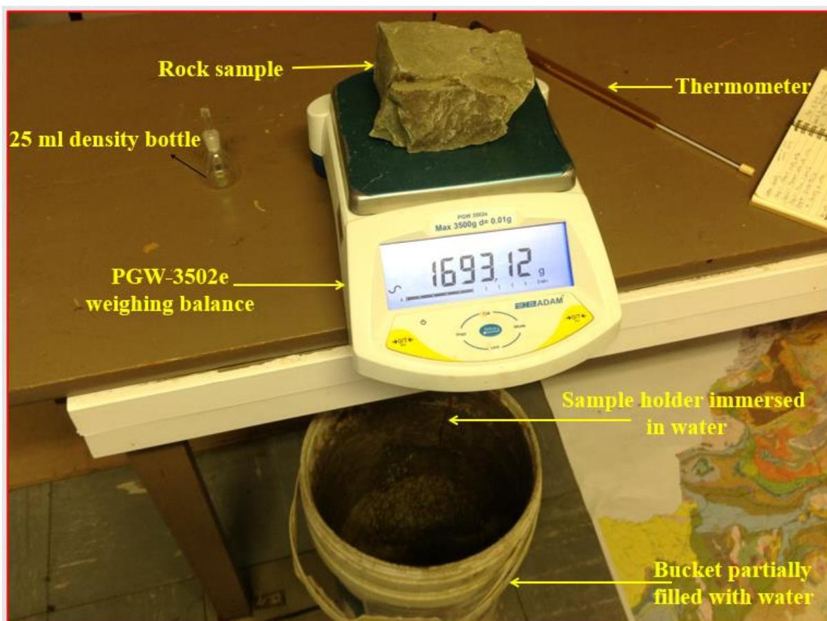
**Figure 3.** Photo demonstrating the use of Archimedes' Principle in rock samples measurement.
