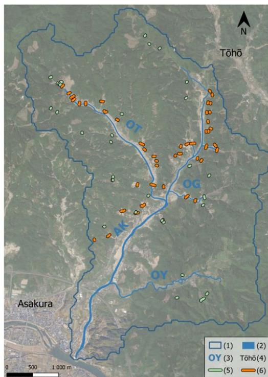
**Figure 6.** ECD constructed in AK watershed before and after 2017. (1) AK watershed area; (2) 2022 channels; (3) hydronym; (4) city name; (5) pre- 2017 dams; (6) post-2017 dams.
