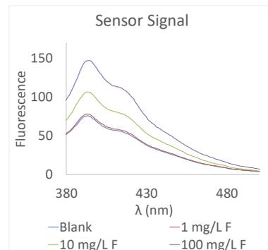
Fluorescence increase (at 398nm) relative to the blank was used as the analytical signal
