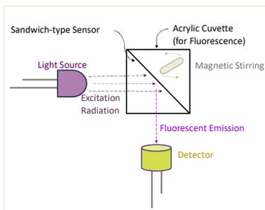
For measurements, the sandwich sensor was positioned diagonally within a fluorescence cell and then filled either with ISO Grade 1 water (blanks) or solutions containing different concentrations of Sodium Fluoride.
