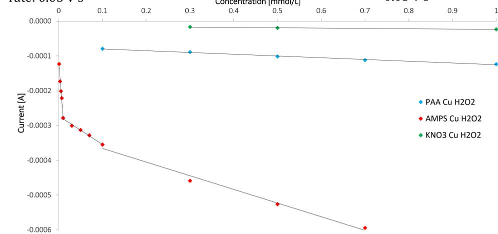
Fig. 4. Calibration curves created for aqueous solutions of supporting electrolytes with a different concentrations of hydrogen peroxide with the addition of copper (II) ions. PAA - blue, AMPS - red,  $\text{KNO}_3$  - green. Measurement conditions: step potential  $-0.005 \text{ V s}^{-1}$ , amplitude 0.2 V, frequency 8 Hz.
