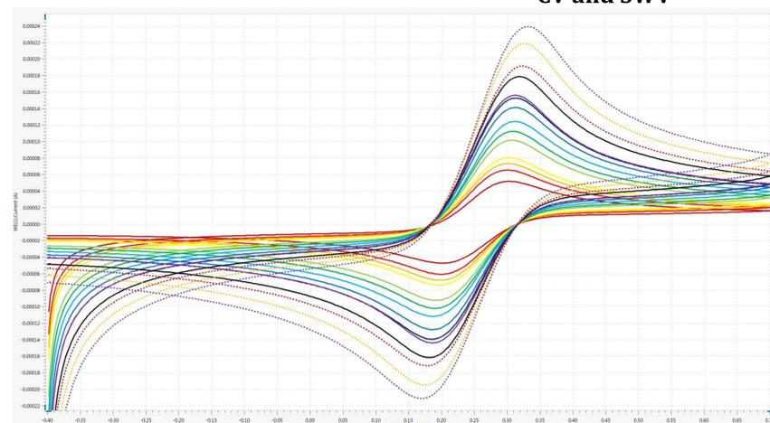
Fig 5. Cyclic voltammograms of peak height versus scanning rate for a 1% PAA aqueous solution in the presence of hexacyanoferrate (II) and (III) ions.
