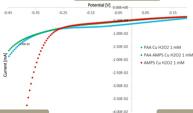
Fig 1. Comparison of square wave voltammograms for solutions: PAA with  $\text{Cu}^{2+}$  ions and 1 mM  $\text{H}_2\text{O}_2$  (blue), AMPS with  $\text{Cu}^{2+}$  ions and 1 mM  $\text{H}_2\text{O}_2$  (red) and a mixture of PAA, AMPS with  $\text{Cu}^{2+}$  ions and 1 mM  $\text{H}_2\text{O}_2$  (green). Measurement conditions: step potential  $-0.005 \text{ V s}^{-1}$ , amplitude 0.2 V, frequency 8 Hz.
