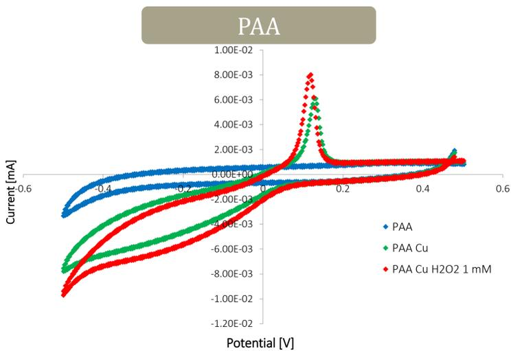
Fig. 2. Cyclic voltammograms for: 1% PAA solution (blue), PAA with  $\text{Cu}^{2+}$  (green), PAA with  $\text{Cu}^{2+}$  and 1 mM  $\text{H}_2\text{O}_2$  (red). Scan rate:  $0.05 \text{ V s}^{-1}$
