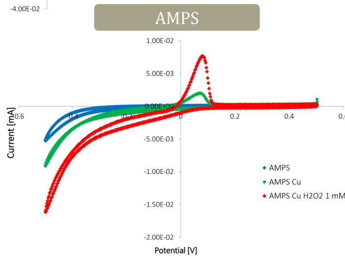
Fig. 3. Cyclic voltammograms for: 1% AMPS solution (blue), AMPS with  $\text{Cu}^{2+}$  (green), AMPS with  $\text{Cu}^{2+}$  and 1 mM  $\text{H}_2\text{O}_2$  (red). Scan rate:  $0.05 \text{ V s}^{-1}$
