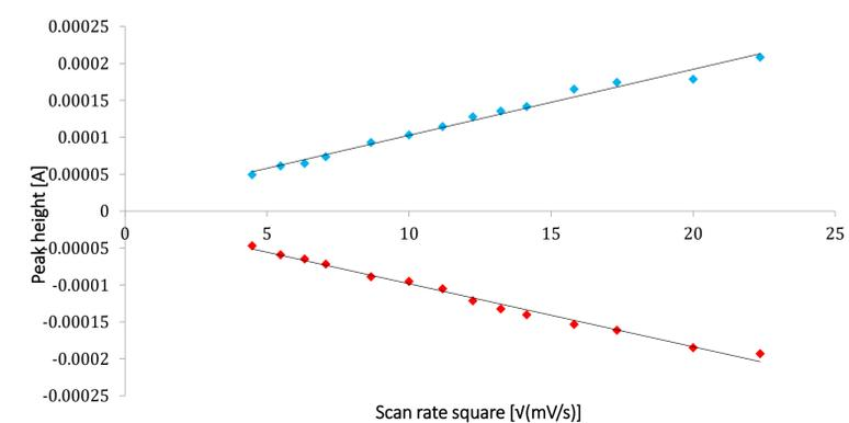
Fig. 6. Peak height vs. square scanning speed curves for hexacyanoferrate (II) ions in a 1% PAA solution.
