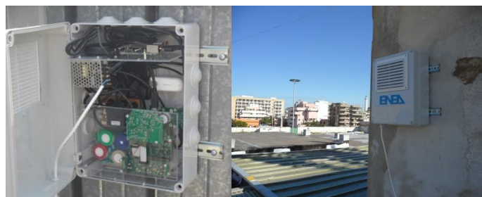
Figure 1. Sensor-node AIRBOX, developed by ENEA, deployed for air quality monitoring.
