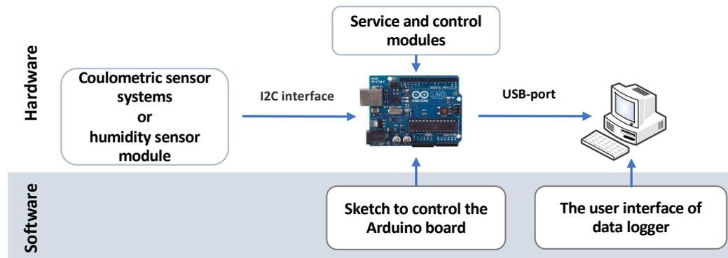
**Figure 1.** A general Arduino-based circuit for electronic data acquisition devices.
