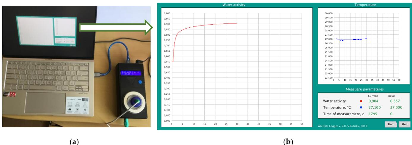
**Figure 2.** An Arduino-based water activity data acquisition device of foodstuff: (a) Photograph of a device connected to a computer; (b) Screenshot of the user interface for monitoring the change in water activity and temperature over.
