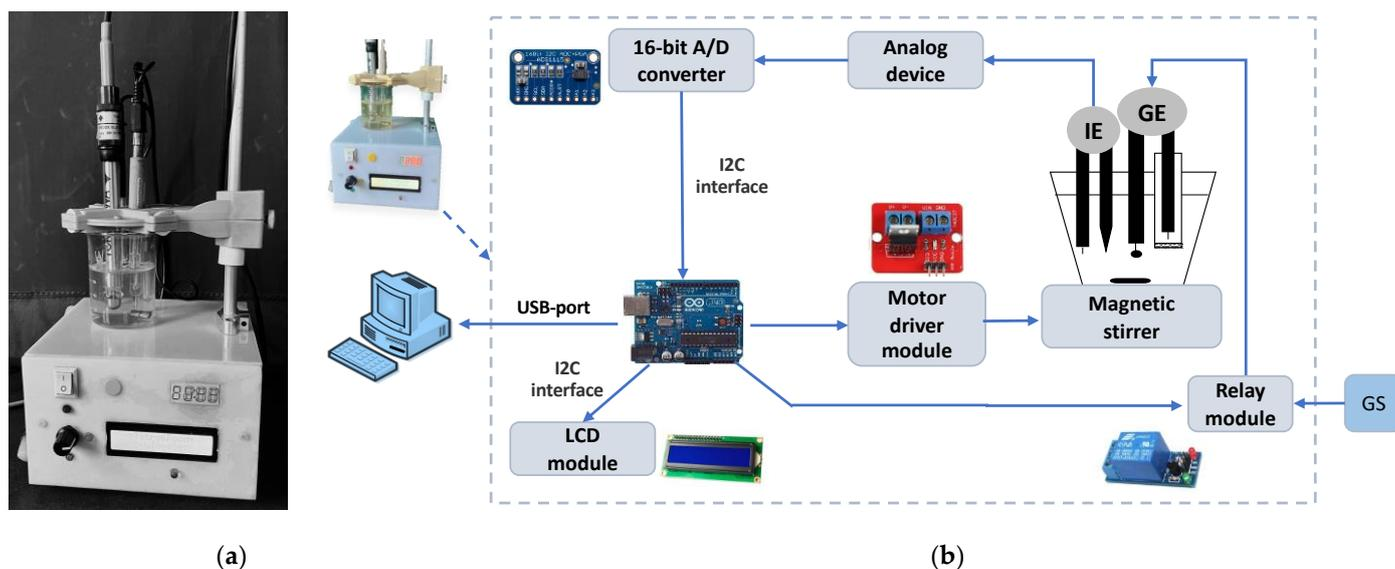
**Figure 3.** An Arduino-based water activity data acquisition device of foodstuff: (a) Photograph of the device; (b) A general Arduino-based circuit for constant-current coulometric titration equipment with potentiometric indication of the titration end point.
