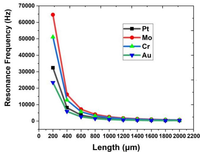
Figure 2. MEMS bridge beam resonance frequency Finite element model for all materials
