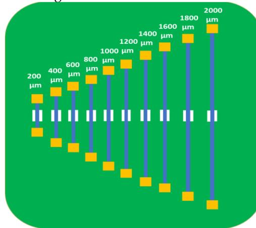
**Figure 1.** An array of designed bridge beam resonators.
