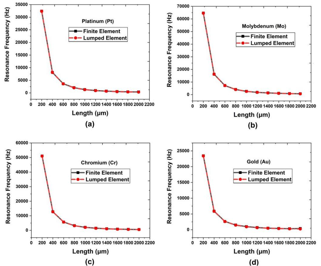
Figure 3. An illustration of the resonance frequency simulated and calculated for MEMS bridge beams made of Platinum (Pt), Molybdenum (Mo), Chromium (Cr), and Gold (Au)
