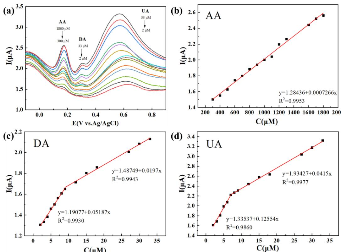
**Figure 2.** (a) DPVs recorded for different concentrations of AA, DA and UA at the  $\text{Ti}_3\text{C}_2\text{T}_x/\text{TiO}_2$  NWs/GCE in 0.1 M PBS (pH 7.4) upon successive additions from 300 to 1800  $\mu\text{M}$  for AA, 2 to 33  $\mu\text{M}$  for DA and 2 to 33  $\mu\text{M}$  for UA,.
