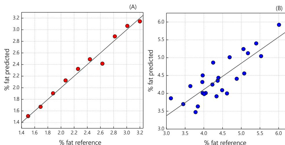
**Figure 3.** PLS-predicted versus reference plot for fat content in: (A) homogenized milk samples and (B) raw milk samples. Red (A) and blue circles (B) indicate cross-validation results.
