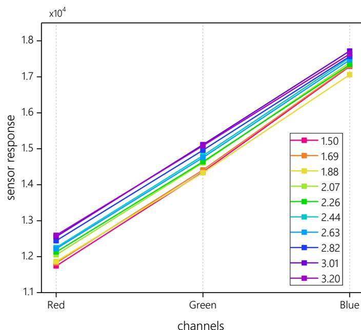
**Figure 2.** The channel responses of LED sensor for dataset of homogenized milk, colored in rainbow gradient depending on fat content (there is a legend of colors on the right side of the plot).
