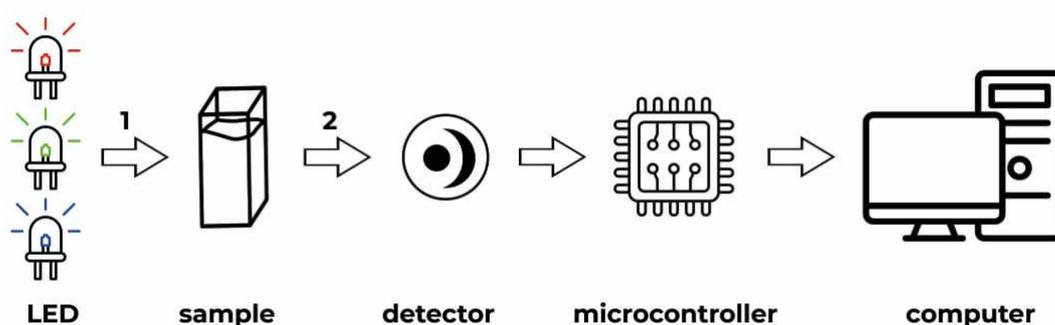
**Figure 1.** Block diagram of the RGB sensor prototype, where (1) designates the emitted light; (2) – transmitted light.
