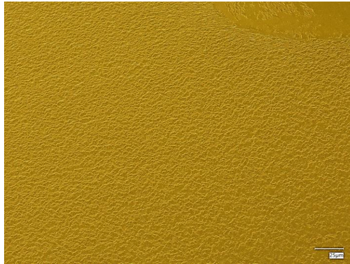
Figure 4. Digital microscope images and roughness profile of hydrogel materials: 1.0 PEG/9.0 PVA (a); 3.0 PEG/7.0 PVA (b); 5.0 PEG/5.0 PVA (c); 7.0 PEG/3.0 PVA (d); 9.0 PEG/1.0 PVA (e).
