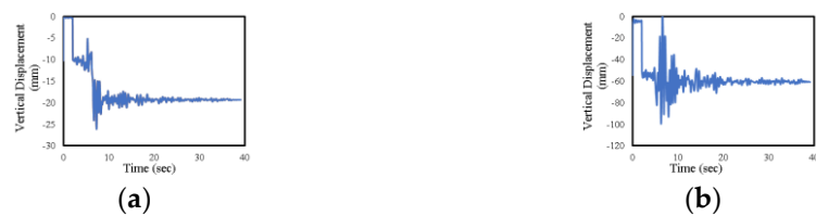
Figure 7. Vertical displacement-time diagrams of the 2-story building models with a: (a) 30 degrees skewed connection and the scenario number 4, (b) 60 degrees skewed connection and the scenario number 3.
