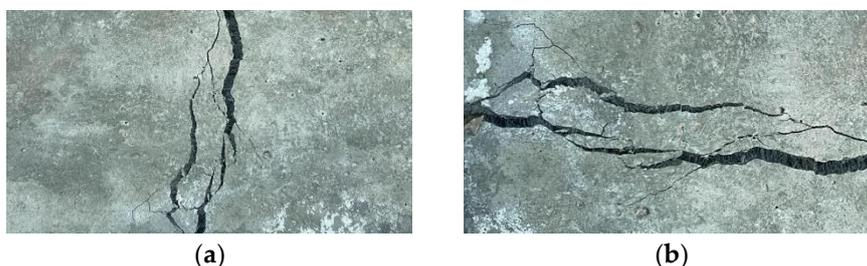
**Figure 3.** Shows the cracking of 2% PPGF-ECC composite: (a) Slab1; (b) Slab 2.
