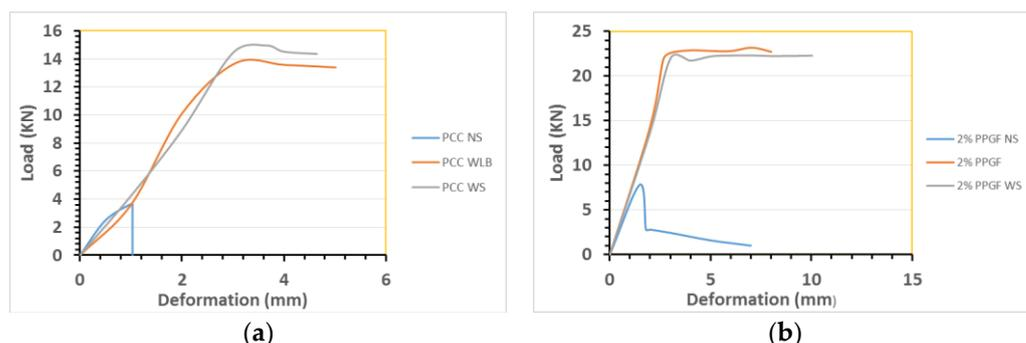
**Figure 2.** Shows the Flexural Behavior of Slabs: (a) PC Slabs; (b) PPGF-ECC Slabs.
