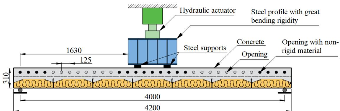
**Figure 2.** Structural configuration used by Braun et al. [6].
