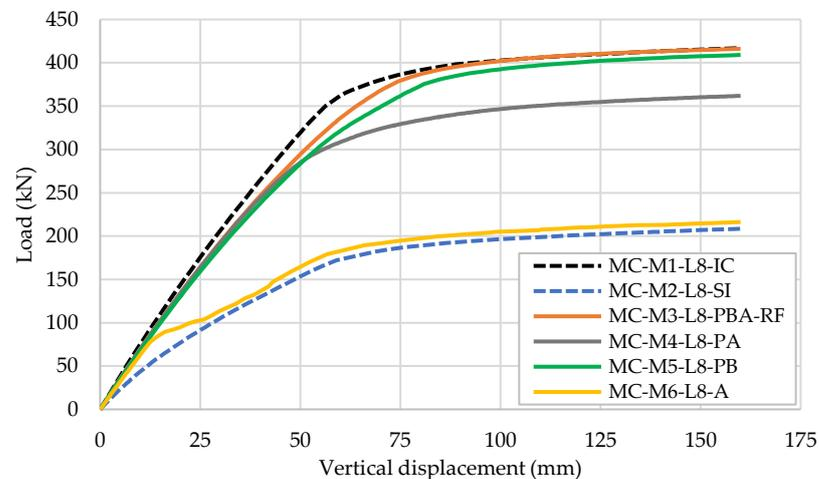
**Figure 6.** Load vs. vertical displacement curves obtained from FE models with different connection mechanisms.
