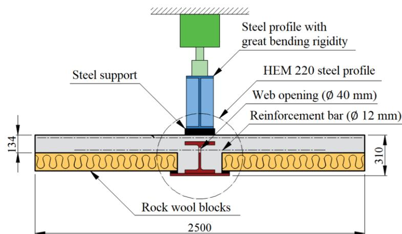
**Figure 1.** Geometric characteristics of the prototypes B1, B2, S1 and S2 experimentally tested by Braun et al. [6].
