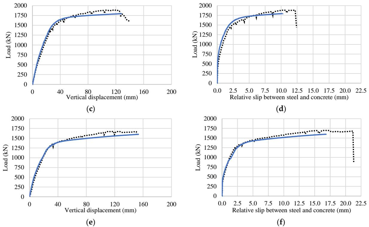
**Figure 5.** Comparison between experimental (dotted black lines) and numerical (solid blue lines) results. (a,b) prototypes B1 and B2; (c,d) relative load vs. slip results of prototype S1; and (e,f) prototype S2.
