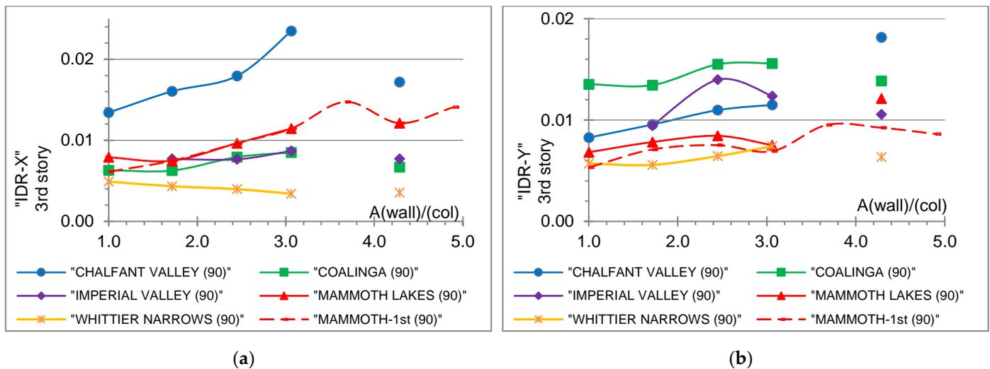
Figure 6. (a) Interstory drift ratio on X axis,  $\theta=90^\circ$ , (b) Interstory drift ratio on Y axis,  $\theta=90^\circ$ , 3rd story.
