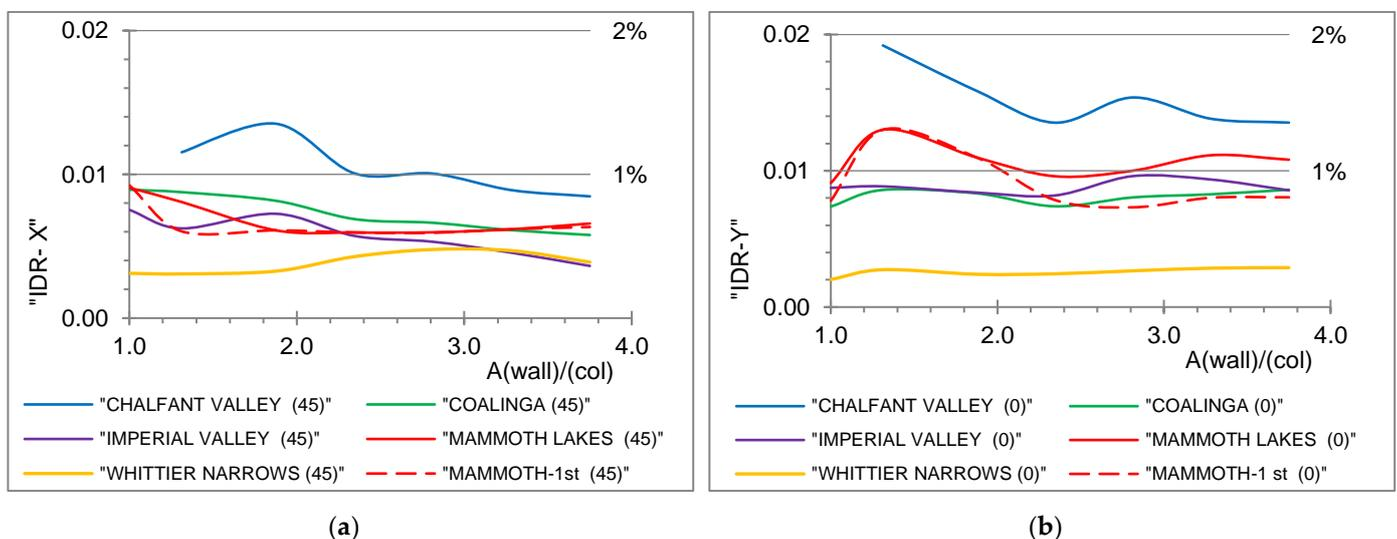
Figure 2. (a) Interstory drift ratio on X,  $\theta=45^\circ$ , (b) Interstory drift ratio on Y,  $\theta=0^\circ$ .
