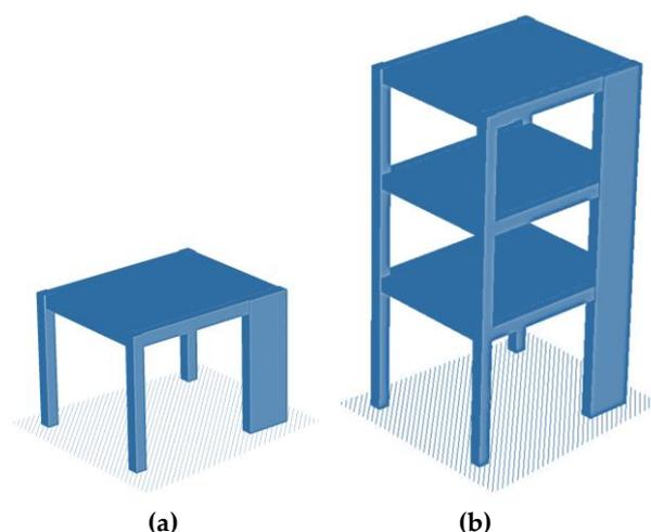
**Figure 1.** Asymmetrical RC buildings with ( a ) one story and ( b ) three stories.
