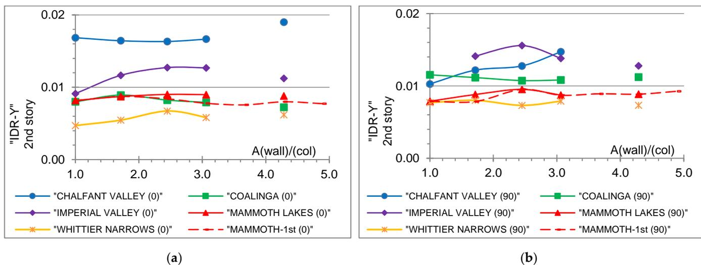
Figure 5. (a) Interstory drift ratio on X axis,  $\theta=0^\circ$ , (b) Interstory drift ratio on Y axis,  $\theta=90^\circ$ , 2nd story.
