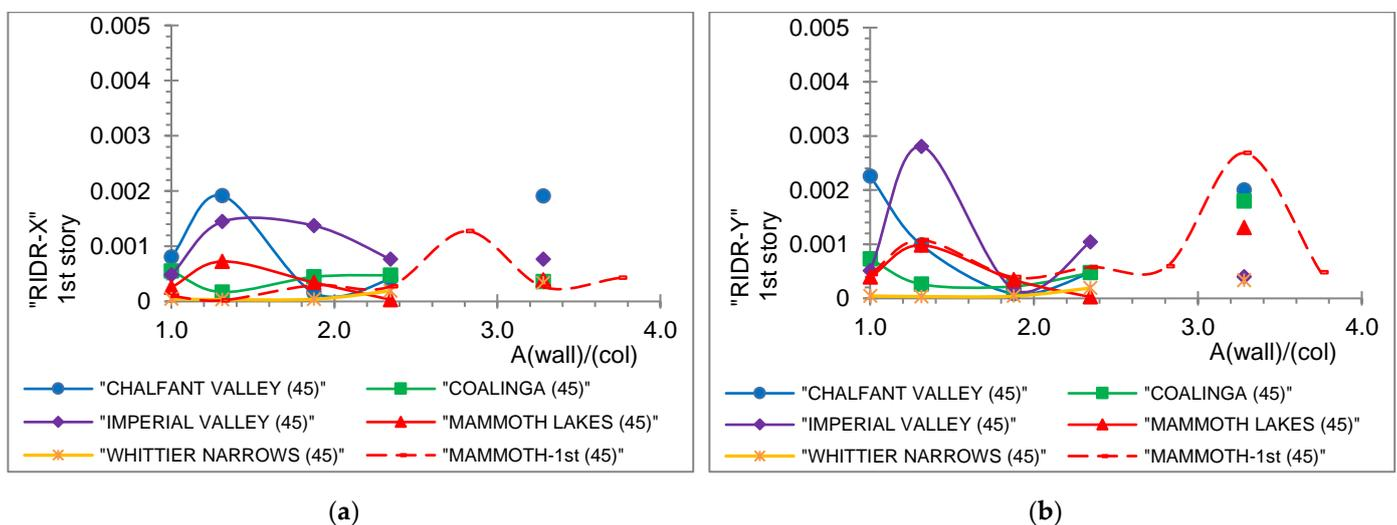
Figure 7. (a) Residual interstory drift ratio on X axis,  $\theta=45^\circ$ , (b) Residual interstory drift ratio on Y axis,  $\theta=45^\circ$ , 1st story.
