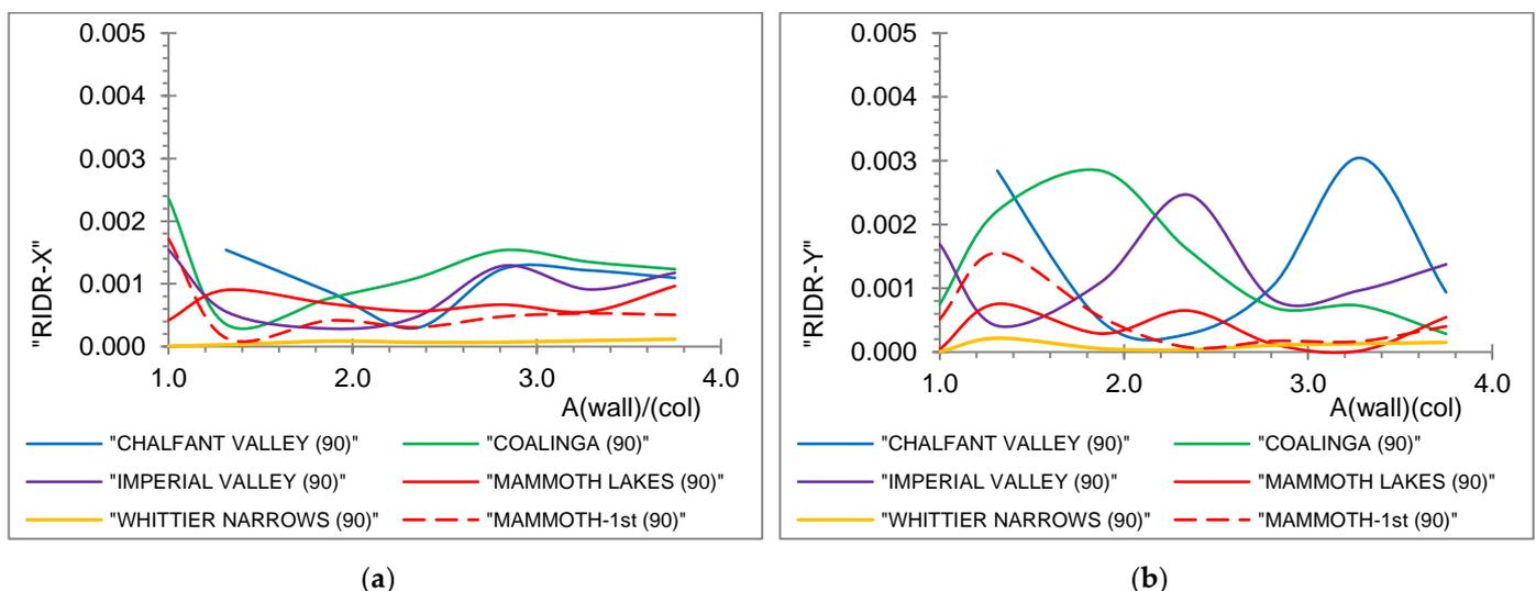
Figure 3. (a) Residual interstory drift ratio on X,  $\theta=90^\circ$ , (b) Residual interstory drift ratio on Y,  $\theta=90^\circ$ .
