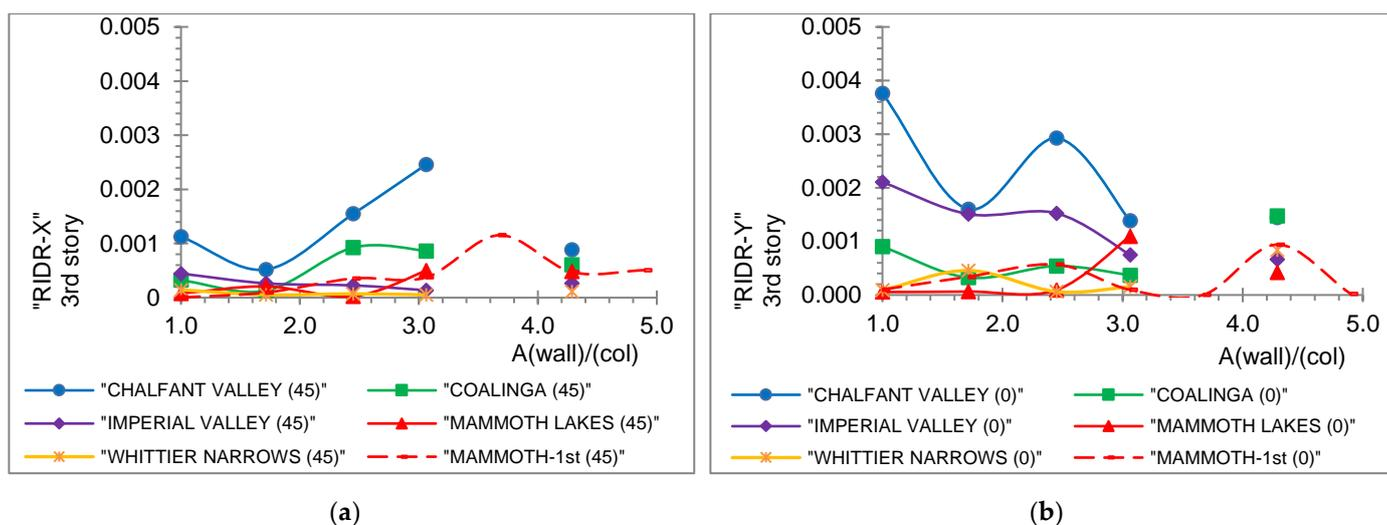
Figure 8. (a) Residual interstory drift ratio on X axis,  $\theta=45^\circ$ , (b) Residual interstory drift ratio on Y axis,  $\theta=0^\circ$ , 3rd story.
