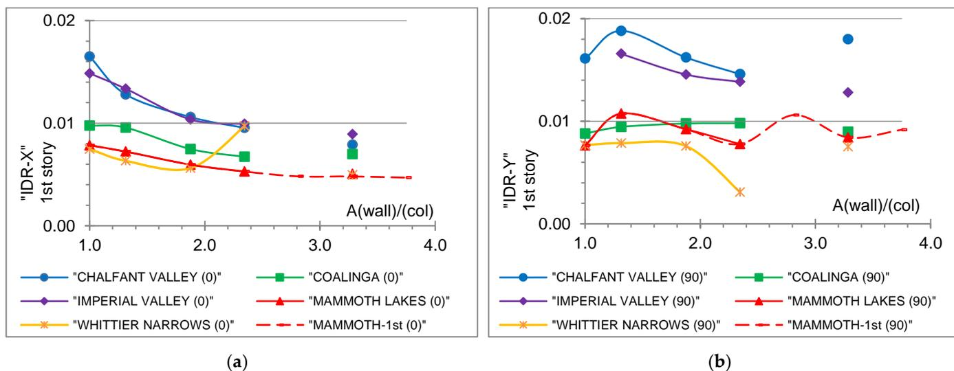
Figure 4. (a) Interstory drift ratio on X axis,  $\theta=0^\circ$ , (b) Interstory drift ratio on Y axis,  $\theta=90^\circ$ , 1st story.
