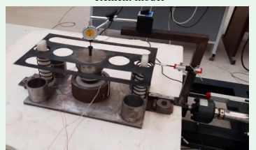
The installed Maglev isolator specimen on the shaking table
