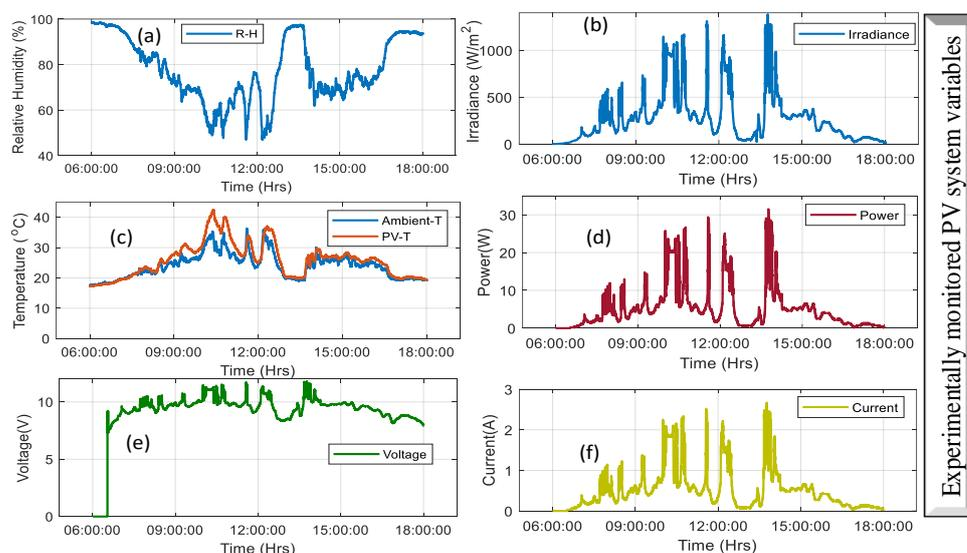
Figure 7. Experimental measurement of the PV system recorded by the Trio-PV-monitor device on a 30 W PV system, 3 September 2023. (a) Relative Humidity (b) Irradiance (c) Ambient Temperature and PV Temperature (d) system Power (e) System Voltage (f) System Current.
