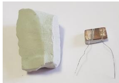
Figure 1. Fabricated NTC-thermistor and starting clinoptilolite mineral.
