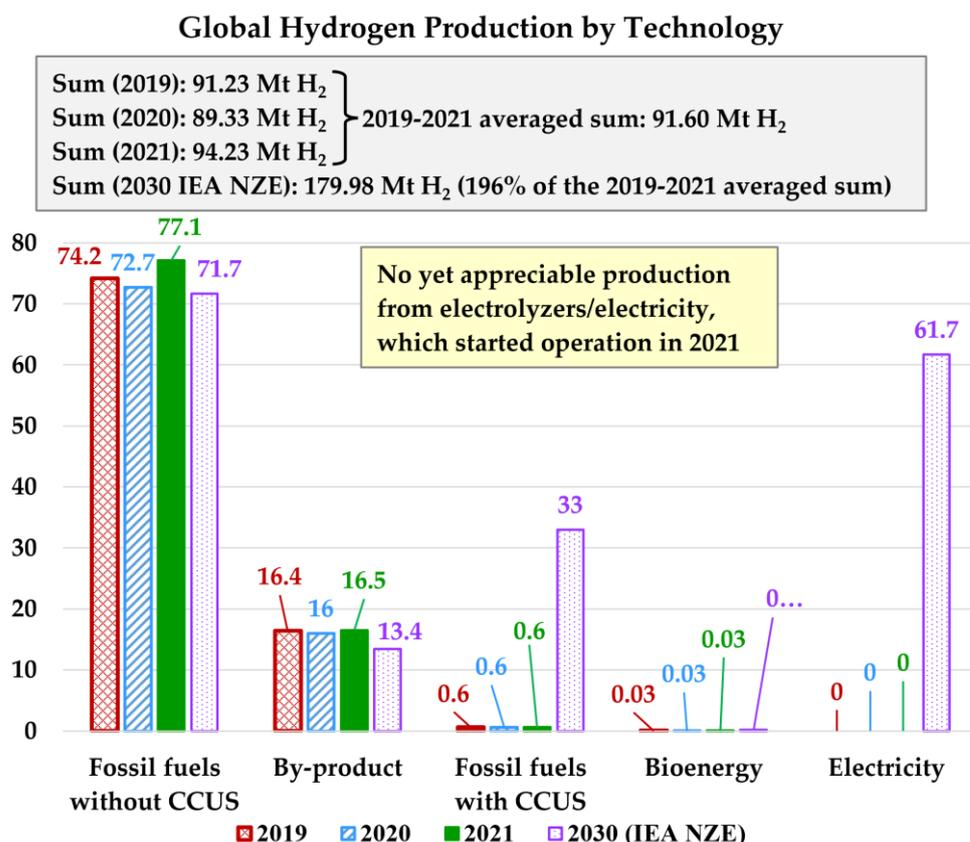
**Figure 1.** Global hydrogen production by source technology, in 2019, 2020, 2021; and the corresponding 2030 expected production according to the NZE of the International Energy Agency (IEA).
