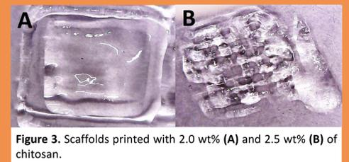
Figure 3. Scaffolds printed with 2.0 wt% (A) and 2.5 wt% (B) of chitosan.
