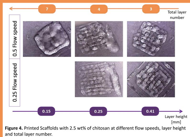
Figure 4. Printed Scaffolds with 2.5 wt% of chitosan at different flow speeds, layer height and total layer number.
