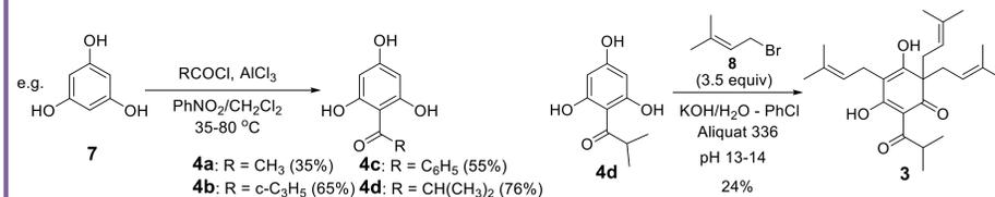
A first series of colupulone analogues 4 was prepared by introducing an acyl group by Friedel Crafts on the phloroglucinol core and colupulone (3) was prepared by incorporating prenyl side chains on the aromatic core by C-alkylation in alkaline conditions [5].
