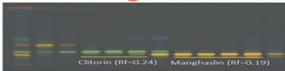
○ The high-performance thin-layer chromatography profile of clitorin and manghaslin fraction under ultraviolet light at 366 nm.
