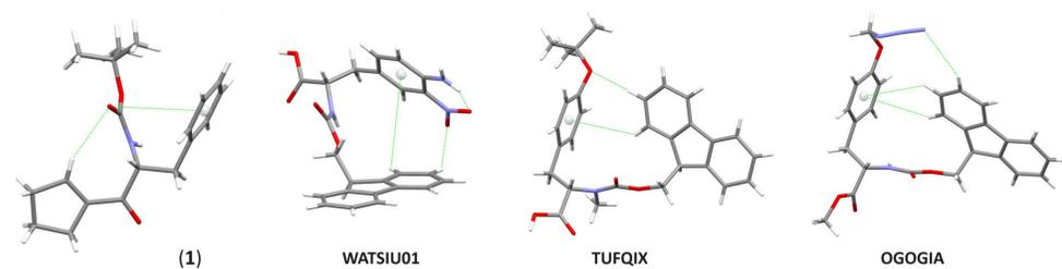
Fig. 1. Pseudo-cyclic motifs created by intramolecular non-covalent interactions and stabilized by interactions involving  $\pi$  electrons. Unique pseudo-bi-cyclic system in (1) *via* intramolecular interactions C-H...O and C-O... $\pi$ . \*WATSU01 [9], OGOGIA [10]
