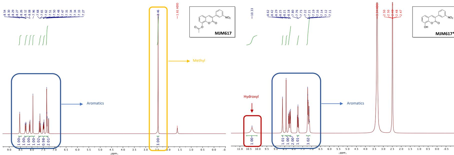
Example of <sup>1</sup>H NMR spectra of a hydroxyl derivative (**MJM617\***) and its acetoxy precursor (**MJM617**).
