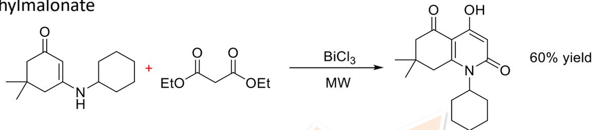
A new, rapid, and environmentally friendly method for synthesizing hydroxyquinolone have being developed
