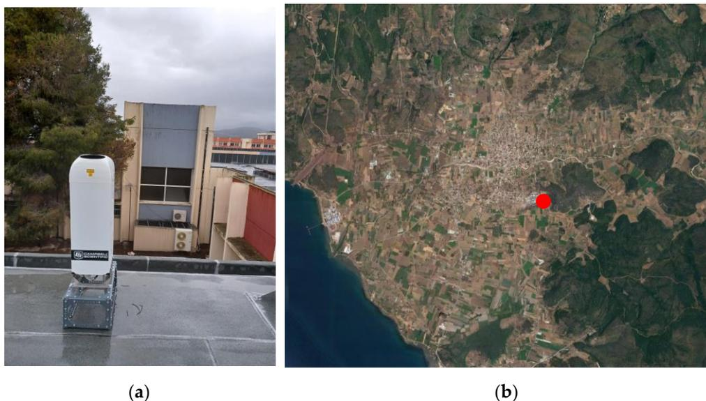
**Figure 1.** (a) Campbell Ceilometer C135 which is operating in the National Kapodistrian University of Athens (Greece), Department of Aerospace Science and Technology in the facilities of Euboea Island. (b) The greater area around the ceilometer (red dot).
