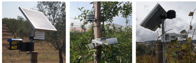
Figure 2. Smart traps installed in olive groove (left), orchard (middle) and vineyard (right).
