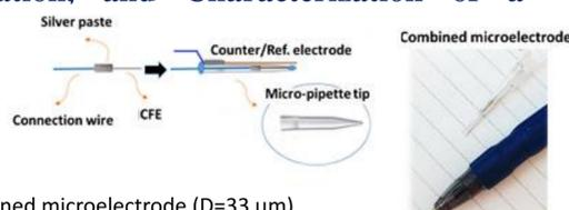
Figure 1. Schematic of fabrication of combined microelectrode (D=33  $\mu\text{m}$ ) and its image.
