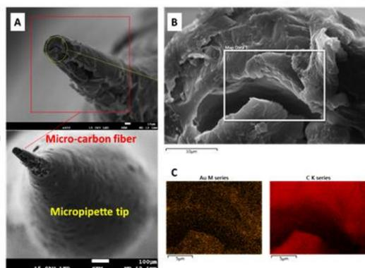
Figure 2. SEM images of modified carbon microelectrode with Au film (CME@Au).
